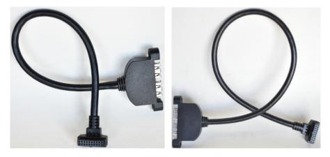
CBG288 shown below with vertical connection to the PCB connector.
