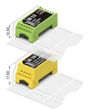
M1 Tibbits are single-width modules occupying one <u>"M" socket on the standard tile</u>. Their footprint is roughly 7 x 14 "squares" (one "square" is  $2.54 \times 2.54$  mm).
