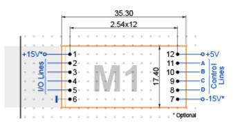
Pins 8-11 are control lines A-D. They are for interfacing to our <u>embedded modules</u> or other microcontrollers. On <u>Tibbo Project PCBs</u> these pins are connected to the main processor.
