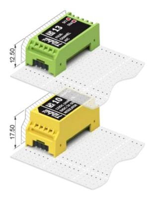
M1 Tibbits are single-width modules occupying one "M" socket on the standard tile. Their footprint is roughly 7 x 14 "squares" (one "square" is 2.54 x 2.54 mm).
