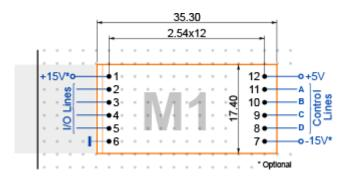
**Pins 8-11** are control lines A-D. They are for interfacing to our <u>embedded modules</u> or other microcontrollers. On <u>Tibbo Project PCBs</u> these pins are connected to the main processor.
