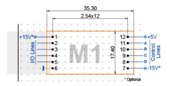
**Pins 8-11** are control lines A-D. They are for interfacing to our <u>embedded modules</u> or other microcontrollers. On <u>Tibbo Project PCBs</u> these pins are connected to the main processor.
