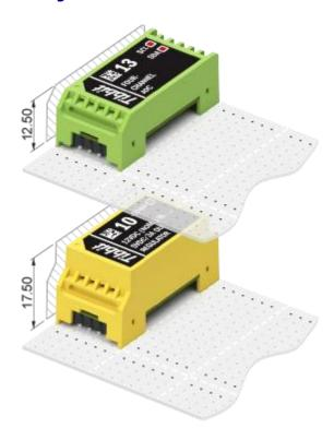
M1 Tibbits are single-width modules occupying one "M" socket on the standard tile. Their footprint is roughly 7 x 14 "squares" (one "square" is 2.54 x 2.54 mm).
