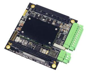
With wide-range input voltages, transient suppression, galvanic isolation, and quick-disconnect terminal mating plugs, this rugged design is ideal for any industrial application.
