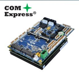
Ideal for space constrained applications, harsh environments, demanding conditions and supports extended temperature ranges of -40°C to +85°C.
