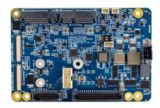
Hadron's design includes a wide input voltage, rich I/O set as well as locking IO connectors optimized for rugged environments.
