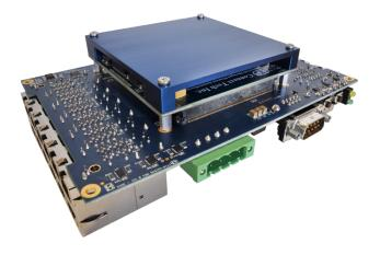
XDG205-01 - XDG205 Switch with XHG201 Heatplate installed Also Shown: XBG301 Development Breakout Board (Sold separately)
